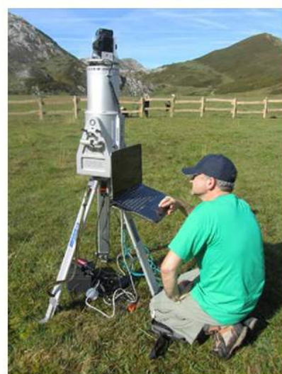
Analysis of possible microtopographical variations to the mire is performed using a laser-scanner.
